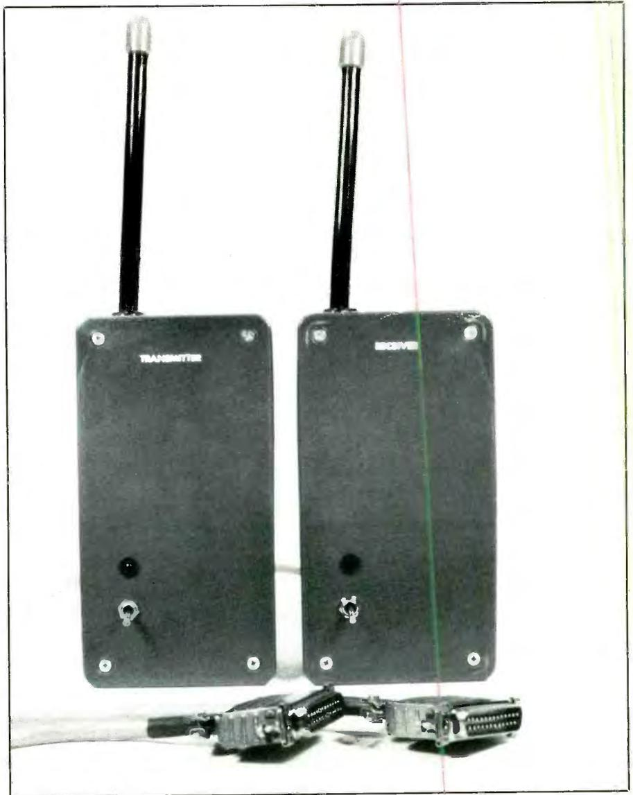
system can accept and generate bipolar RS232-compatible signals, at a communication speed of 300 bits per second.
