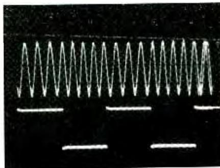
Fig. 3. The bottom trace shows the digital RS232 signal. The top trace is the frequency-shift-keyed output at the modem chip.
